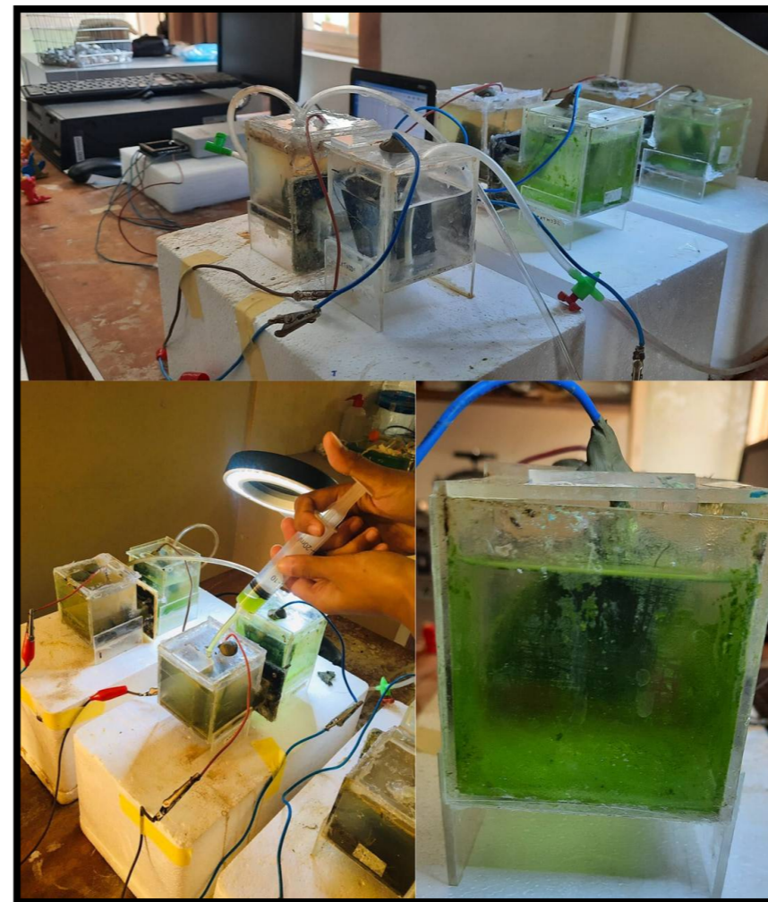
Figure 6. Several different photosynthetic microbial fuel cell (PMFC) types used at the MEU of Rajarata University, Sri Lanka to investigate fully sustainable and cost-effective utilization of MFC systems.
